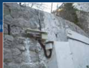
Extensimeters with cable on the surface
